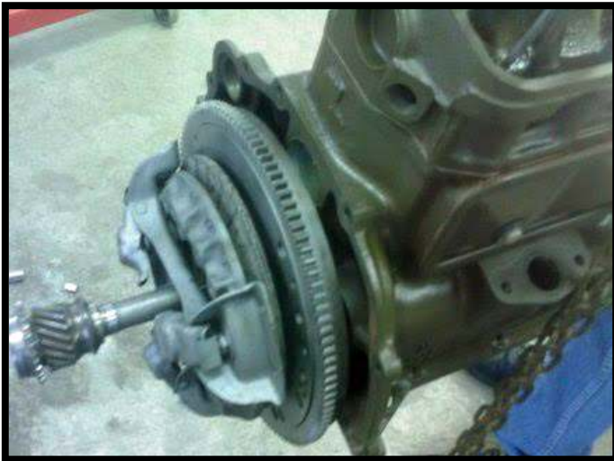
15. Lastly, the clutch assembly is installed.
