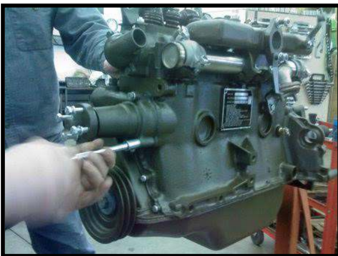
13. Continuing with mounting the water pump
