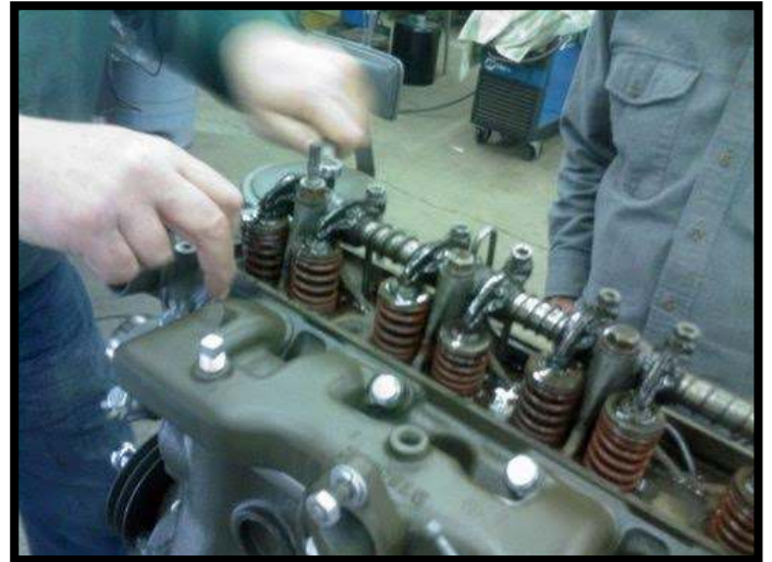
10. Brant starts the process of adjusting valve clearance
