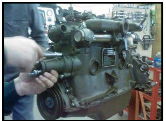
12. Installing the water pump
