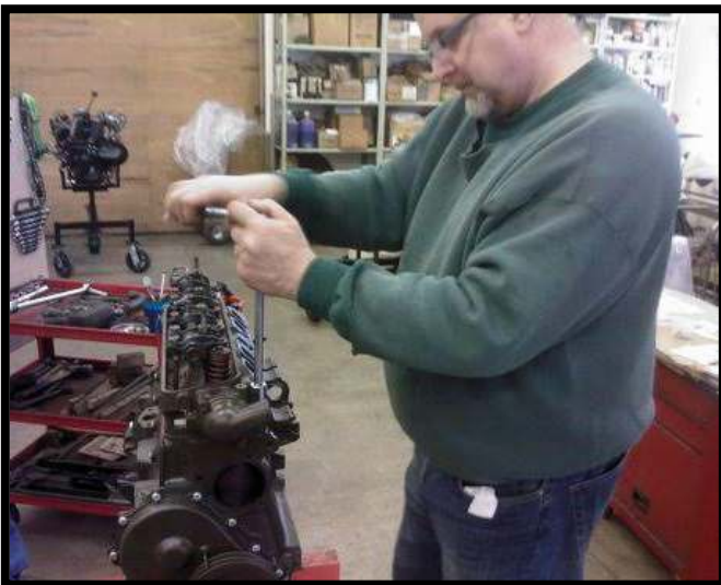
5. Using a torque wrench, Brant secures the head
