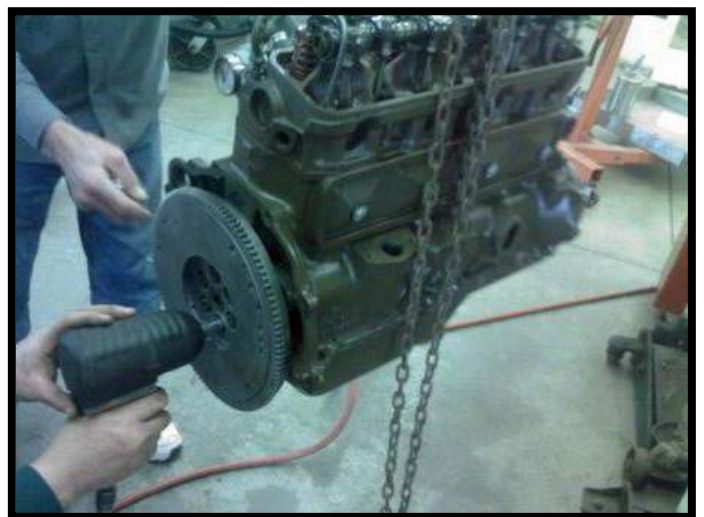
14. Installing the flywheel
