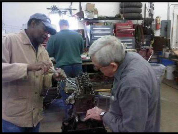
9. Tighten up the manifold bolts.
