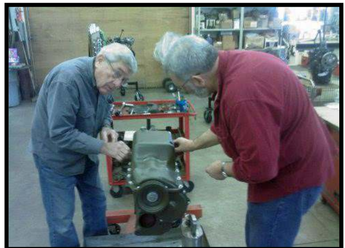
2. Bob and Scott install the oil pan
