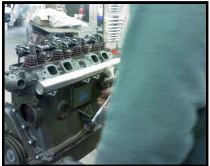
6. Installing a manifold
