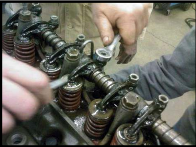
11. Brant continues the process of valve clearance
