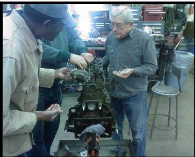
7. Securing intake manifold for mounting
